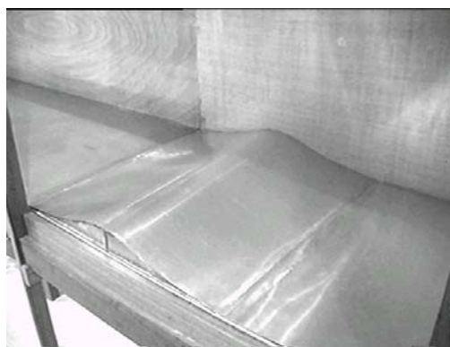
Figure 31. Model of the hill inside the wind tunnel.
