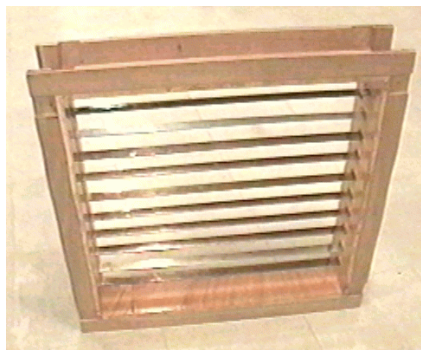
Figure 30. Stratification section of the wind-tunnel.
