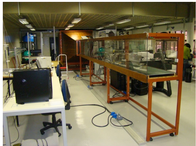
Fig. 5 Open circuit blower-type wind tunnel of DINAM-INMETRO
