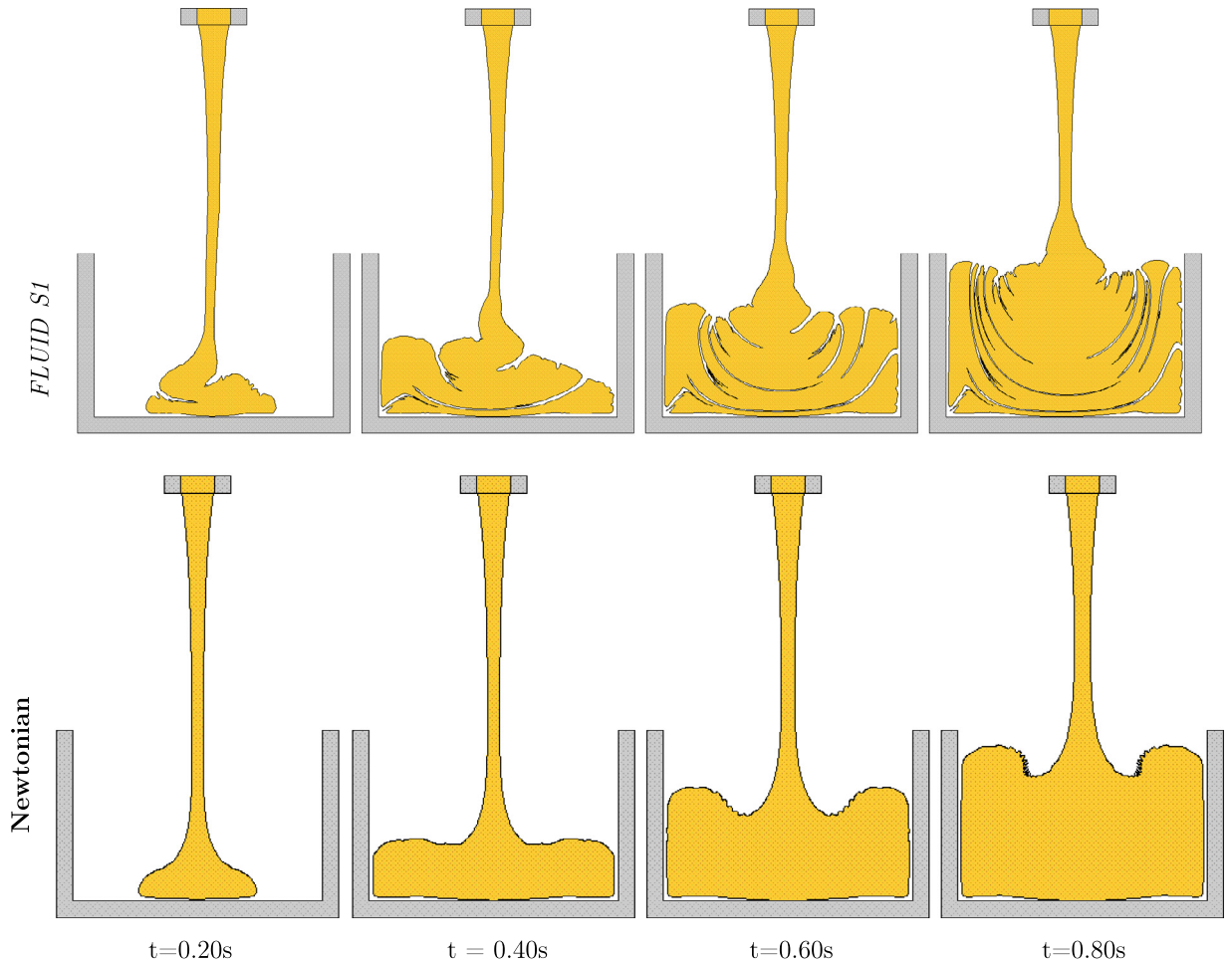
Fig. 20. Numerical simulation of impinging Newtonian and FLUID S1 jets with U = 0.28 \text{ m s}^{-1} . Fluid flow visualization at selected times.
