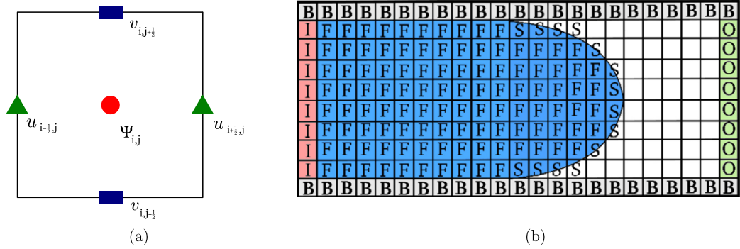
Fig. 1. (a) Typical two-dimensional staggered cell. (b) Illustration of cell type classification used.
