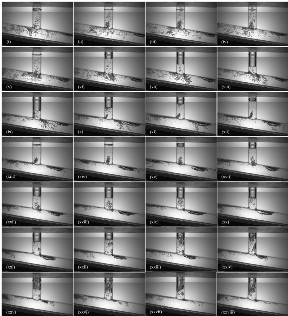
Fig. 4 Dynamics of bubble separation at the T-junction: high speed images for experimental condition EB2 (elongated bubbles). Frequency of acquisition is f_{aq} = 250 Hz. Time interval between the above images = 10f_{aq}^{-1}
