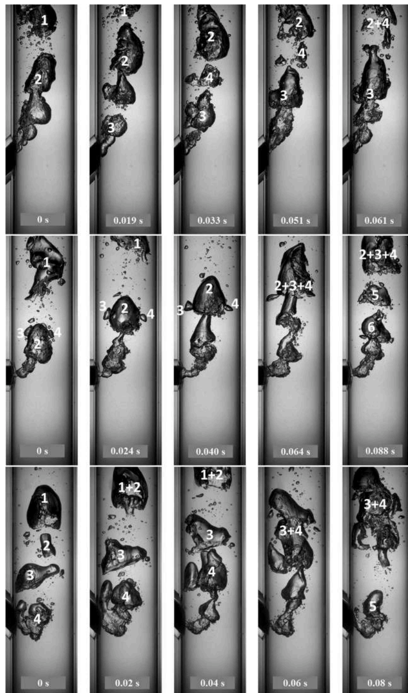
Fig. 5. Flow patterns for d_{inj} = 2 mm, Q_L = 2 m 3 h -1 , Q_G = 0.57 m 3 h -1 and the three injection angles: \gamma = 45^\circ , 0^\circ and -45^\circ .
