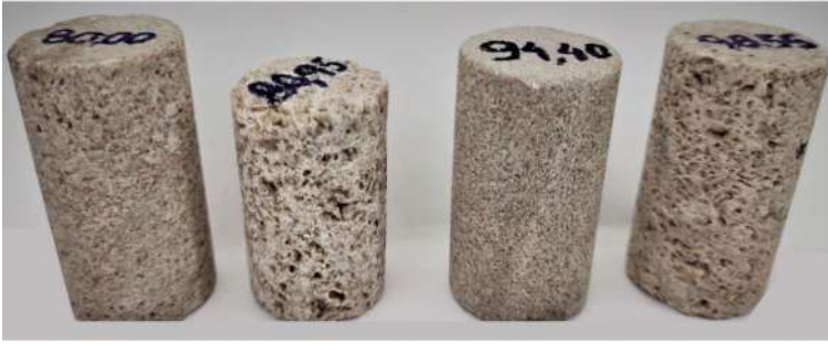
Fig. 1 Samples used in this study showing different apparent textures and pore structures at their surfaces
